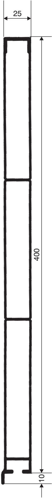
HP16 One Piece Dropside System Drawn half size
